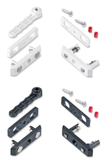
The tappet contacts ST9121 (white) and ST9122 (black) are suitable for transmission of electricity to windows or doors. A permanent electrical contact stability is ensured by a strong magnet that attracts the magnetic tappets. This contacts work entirely without access ramp, which allows the contacts to close from each position and side. As a result, the contacts are qualified for both normal window, turn/tilt doors as well as for lifting/sliding doors.
